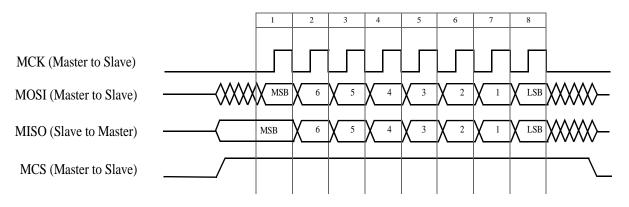
Note: MCS shown terminating after one byte for illustrative purposes only, actual transfers must maintain MCS in the active state for one frame of 9 bytes.
