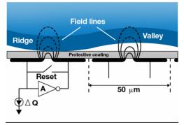
Figure 2: Principle of Operation
